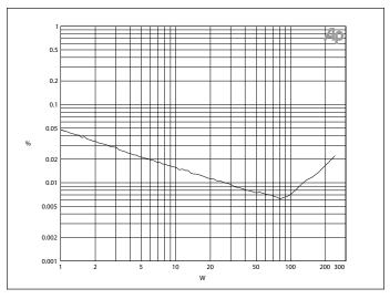
THD+N vs Output Power. Bandwidth limited to 10 Hz - 22 kHz
