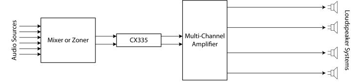
The CX335 is normally connected into the audio system between the mixer, zoner or other sound source selection component, and the main power amplifiers. The connection is entirely straightforward; the active audio source feeds the CX335's inputs, and its outputs feed the power amplifiers' inputs. All interconnections are stereo, and
