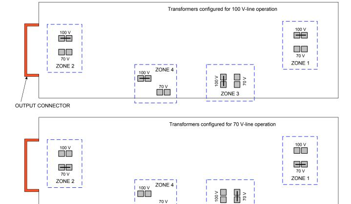
SOLDER SIDE OF PCB, SHOWING APPROX. LOCATIONS OF WIRE LINKS
