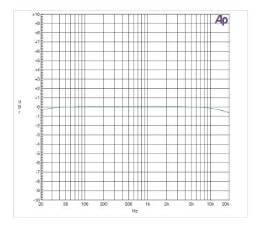
VTX 4400 ES 2 Typical Crosstalk, 4 Ohm load, 400W Output
