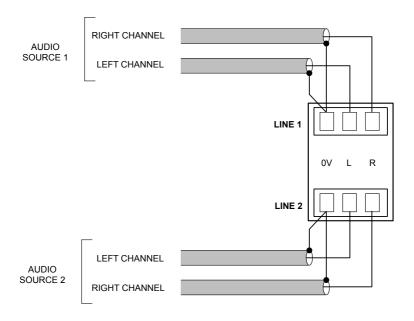
Unless a Cloud remote control plate or module such as the RSL-6 or LM-2 is in use, the two line inputs are summed together internally, though Line input 1 can be configured to have priority over Line input 2, see "Line 1 Priority" on page 19.
