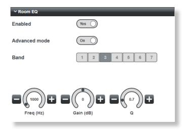
The Q control adjusts the bandwidth of the peaking filter over a range of 0.3 (broad) to 3 (narrow).
