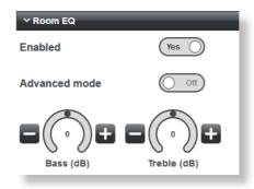
In Basic mode, simple treble and bass shelving filters are provided. The controls have a range of +/-12 dB at frequencies of 10 kHz and 50 Hz respectively.
