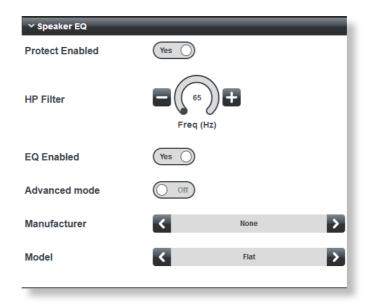
In this mode, it is possible to select a specific loudspeaker EQ preset from a set that has previously been installed. Installation of loudspeaker presets is via a firmware update.
