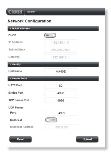
This page displays the network settings for the MA40E. The current IP Address, Subnet Mask, Gateway address and Unit Name are confirmed. If DHCP is set to On, the values in IP Address, Subnet Mask and Gateway are set automatically and the fields greyed out. If assigning these values (with DHCP set to Off), ensure that a suitable, reserved static IP address is used. This may require consultation with the network administrator.
