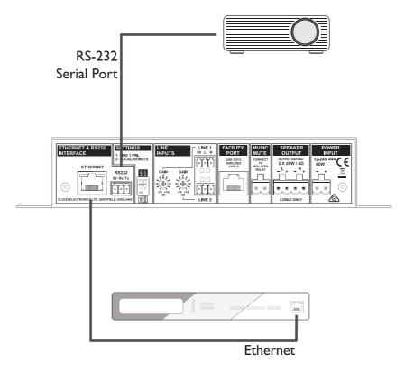
This function uses the MA40E's virtual CDI port, whose address has the default value of 4998. If the controlling device is only able to support remote ports in a certain address range (i.e., not including 4998), the port address can be changed on the Network Configuration page of the browser interface (select Config > Network).
