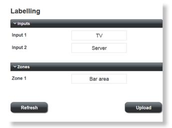
The Labelling page allows the Installer to change the names of the line inputs and the area covered by the amplifier (the default "Zone 1"). Names entered on the Labelling page will replace the default names on all browser pages where they appear. This provides a much more intuitive interface for both Installer and Users.
