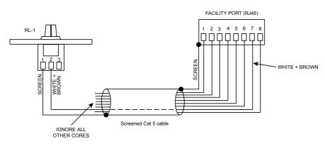
RL-1 REMOTE LEVEL CONTROL WIRING
