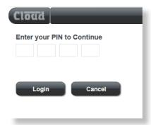
The first page to be displayed on initial connection will be the PIN entry page; enter the Installer PIN (the factory default is 1234¹) to authorise access. Click Login and the Zone 1 page² will be displayed, with the Input Routing and Output tabs open as shown on the following page.
