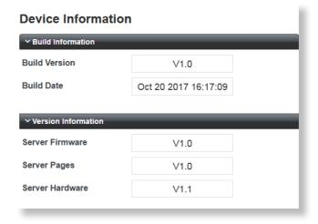
This is an "Engineering" page which gives details of the versions of the various firmware elements in the MA40E.
