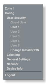
The MA40E security system allows up to five Users - in addition to the Installer - unique PIN access to the control pages. Additionally, a Guest User may access the control pages without a PIN. Clicking on any of User 1 to User 5 opens the User privileges page for that User, as seen on the following page.
