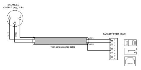
An unbalanced source may also be connected; the use of balancing transformers is recommended.
