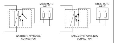
Note that any signal applied to the MPA MK2's Facility Port – either from a remote active module, or as a hard-wired direct input, will be also muted by the action of Music Mute.
