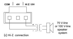
When driving 70/100 V-line loudspeaker systems there is a risk of transformer core saturation at high levels and low frequencies, which can produce distortion. To prevent this, the MPA MK2's output stage is provided with a 65 Hz high-pass filter, which may be enabled by setting **SPEAKER SETTINGS** switch SW1 to on (SWITCH down).
