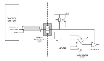
NOTE: If the control voltage source is not isolated from the power earth, there is a small risk of creating a 'ground loop' by linking the mixer technical ground (0 V) to the ground (0 V) of the equipment supplying the control voltages. To minimise this risk, we suggest that all pieces of equipment be in close proximity, and supplied from the same power outlet.
