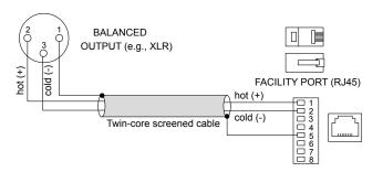
An unbalanced source may also be connected; the use of balancing transformers is recommended.
