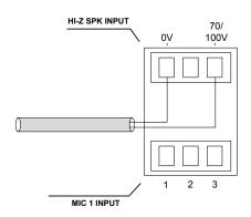
Note that the 70/100 V input is suitable for use with either 70 V-line or 100 V-line systems. The **GAIN** control may be used to adjust for the 3 dB difference in level between the two systems.
