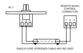
REMOTE SOURCE & LEVEL CONTROL WIRING
