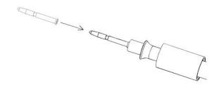
(4) Thread the coaxial cable forward into the BNC male plug after pressing the pin firmly
