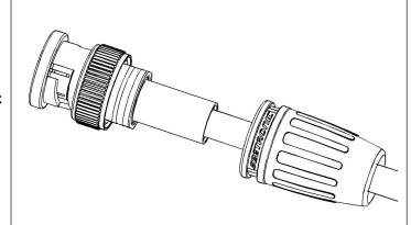
(6) Push the boot assembly forward, buckle into the BNC male connector and the assembly is completed
