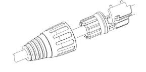
(2) Assemble the cable with RJ45
