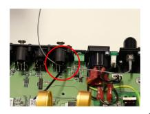
**6.** Push the nylon standoff into the mounting hole. Mount the WiFi module and make sure it snaps into place.
