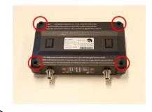
**3.** Remove the cover plate using the T10 screwdriver and the plier. Save the screws and
