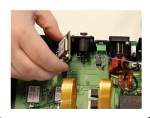
7. Connect the antenna cable to the WiFi module.
