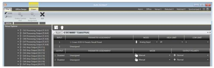
Figure 53: The current preset has been assigned for recall via Control port Input 1
