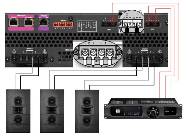
Figure 59: System wiring in Dual mode
