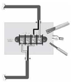
Figure 6: Wiring output connectors
