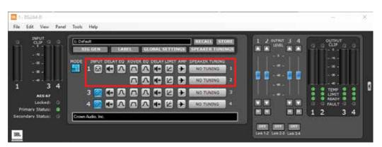
Figure 42: With the "Y 1+2" box checked, both output Ch.1 and Ch.2 are fed by input Ch.1 and input processing is organized accordingly
