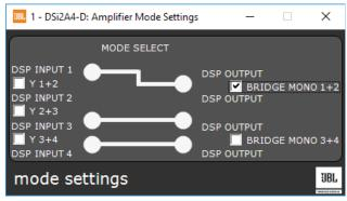
Figure 60: Audio Architect amplifier mode settings
