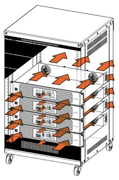
Figure 1: Proper rack venting
