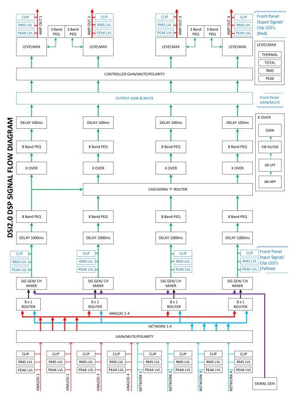
Figure 69: Signal path block diagram (A4-D model Shown)
