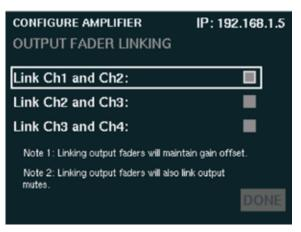
Figure 21: Output Fader Linking screen
