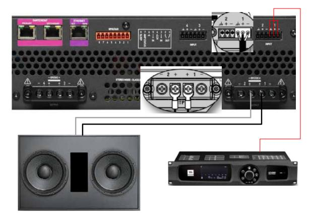
Figure 61: System wiring in Bridge Mono mode
