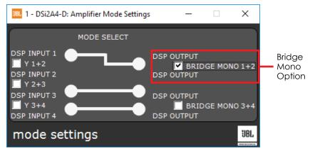
Figure 43: Bridge Mono Configuration
