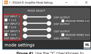
Figure 41: Use the "Y" checkboxes to cascade input channels
