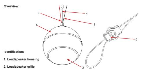
**3.** Loudspeaker cables - Use these cables to connect to your mixer amplifier. Cable colour code: Red = 15W, Yellow = 7.5W, Green = 3.75W, Blue = COM.
