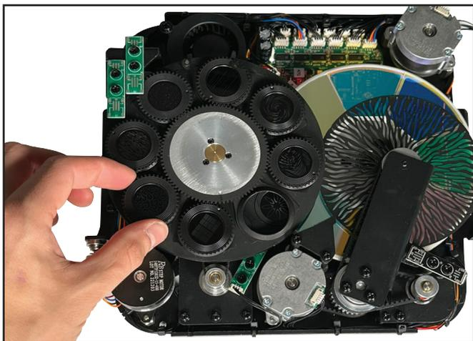
9) Locate the gobo that will be replaced. Grip the edges of the gobo holder and carefully lift the holder until it is raised from the surface of the gobo wheel. Pull the gobo holder towards you, away from the gobo wheel.
