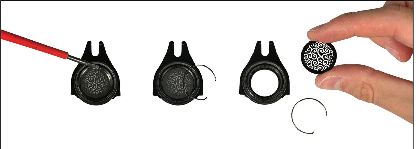
10) Place the gobo on a flat surface with the gear side down. Locate the tab of the spring clip using a precision pick (or similar) and push the spring clip inwards to release it and remove the spring clip. Carefully remove the gobo from the holder avoiding scratching the gobo. Install the new gobo and follow the previous steps in reverse order.
