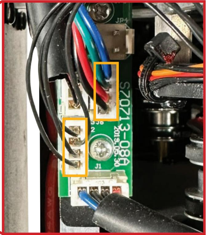
4) To the left of the gobo/colour wheel module there is a sub pcb. Disconnect the framing module connector along with the gobo/colour wheel module connector highlighted in orange above.
