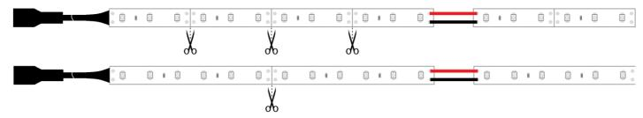
Each 5m reel of single colour LED tape is fitted with a 2.1mm DC jack socket for power input for easy connection to a power supply. This connector may be removed and stripped for bare wire connection if a 2.1mm jack is not fitted to the power supply.
