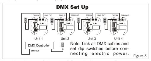
Do not supply power before the whole system is set up and connected properly.
