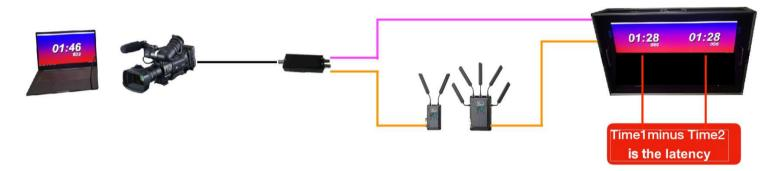
4.3 The audio and video are out of sync when video is directly transmitted to the control room, but audio is transmitted to the control room through an audio mixer.
