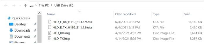
3. Connect the USB disk to the device, and the upgrading process will automatically begin after the restart of the device
