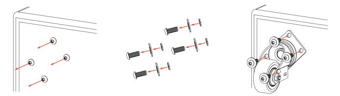
Note: Apply a torque value of 3.9 Nm (35 in-lb) and non-permanent thread lock.
