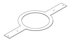
Figure 1: Optional NC New-Construction Bracket
