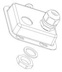
Figure 6: Affixing gland nut to Terminal Cover Plate
