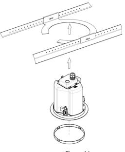
Figure 14: Inserting Speaker into Ceiling
