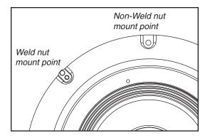
Next, using 4 pcs -  $\#10 \times 0.75$  in (19 mm) sheet metal screw, attaching the baffle / driver to the back can. Be sure to match the mouting holes <u>without</u> weld nuts to clip nuts on back can.
