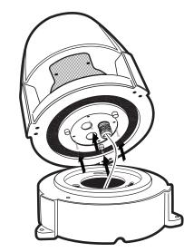
Begin to re-assemble speaker by taking care to place wire nut connectors in top section of speaker and reattach the seal plate with screws as shown above.
