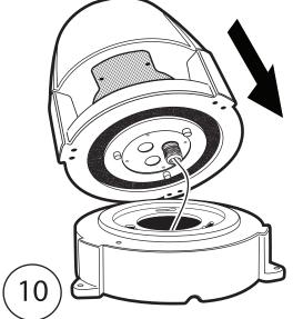
Line up the upper section pins and lower section grooves.
