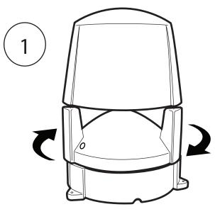
Twist the top part of the enclosure in a clock-wise direction until it disengages from the bottom part.
