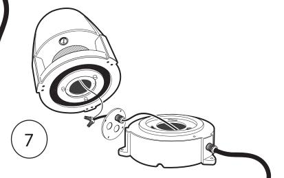
Continue to extend external wire up through the gland nut installed on the seal plate and attach to pre-existing wires from the top section of the speaker with included gel-filled wire nuts.
