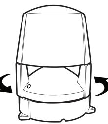
Rotate top section counter-clockwise to lock the top to the bottom section, being careful to line up the security screw hole with brass nut on the bottom half of the speaker.
