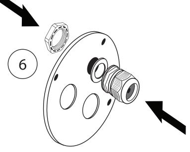
Install the gland nut into the hole as shown
