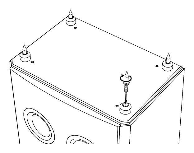
When using the spikes, do not remove the rubber feet from the speaker. To install the spikes, position the speaker on a carpeted or padded surface. Insert the threaded end of the spike into the aperture of the rubber foot. Turn the spike in a clockwise direction and continue until the spike is inserted as far as it will go.
