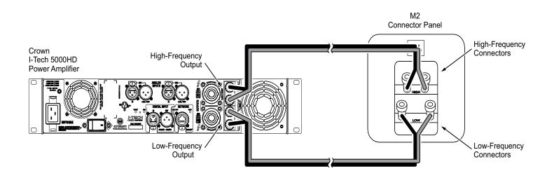
The M2 speaker terminals are designed to accept bare wire. Push down on the top of the terminal to open the connection hole, insert the bare wire and release the terminal to secure the wire.
