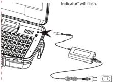
B. Plug the TG-10T/TG-10R into "Charger Slot" of TG-10CH36/TG-10CH18. The "Charging Indicator" will flash for seconds at beginning for initial testing, and then shows green light when charging. It will turn off when the battery is fully charged.
