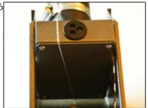
When correctly installed, the wire should be tight like this.
