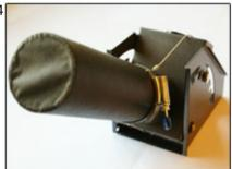
Pull the jubilee clip up the cartridge to tension the wire and tighten.
