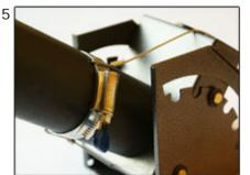
Tighten the clip as tight as you can without deforming the tube, the wire loop will press into the tube this is ok.
