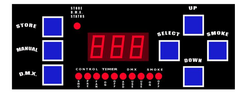
The 'SELECT' button will sequentially cycle through all the adjustable controls.
