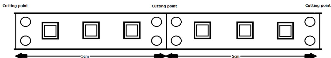
You may also reconnect the two pieces by soldering the connection points together (FIG 2). The tape has two tracks for the DC voltage with + positive pole at the top and – negative pole at the bottom.
