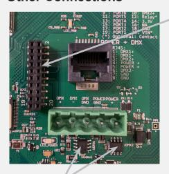
DMX CHIPS To replace, solder the DMX chips to the 8 pin connectors.
