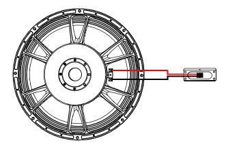
→ To wire eLS18, slit the membrane of the grommet crosswise, pass the cable through and make the connection to the screw terminals. Place the IPCOV.
