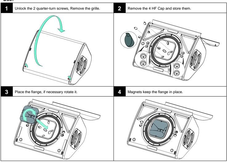
When replacing the grille, ensure it is well positioned in the top blade before fasten with quarter-turn screws.
