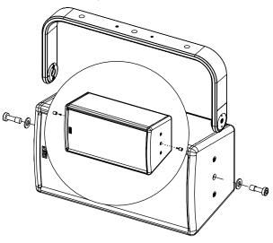
Place on CLADAPT, use the 2 guides. Tight with the fasteners provided with CLADAPT.
