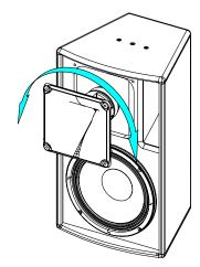
Reassemble the assembly and replace the grille.
