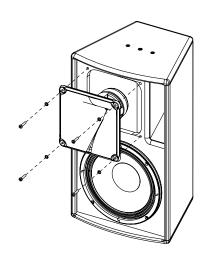
Position the horn according to the desired HF dispersion.
