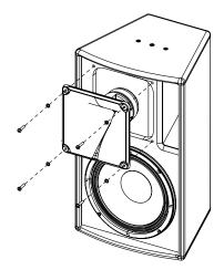
Reassemble the assembly and replace the grille.
