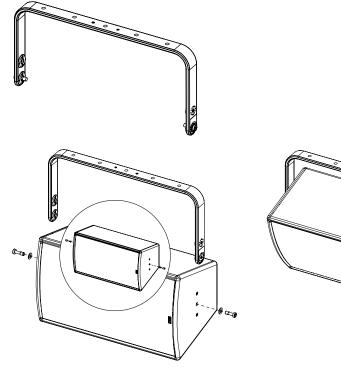
Remove the M10 inserts from each side. Place HBRK535 on ePS10, use only fasteners provided. Tight properly.
