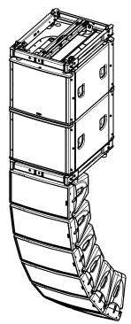
o For long throw stacking application, up to 6 GEOM10, crossover 85 Hz is recommended (also for GEOM10).
