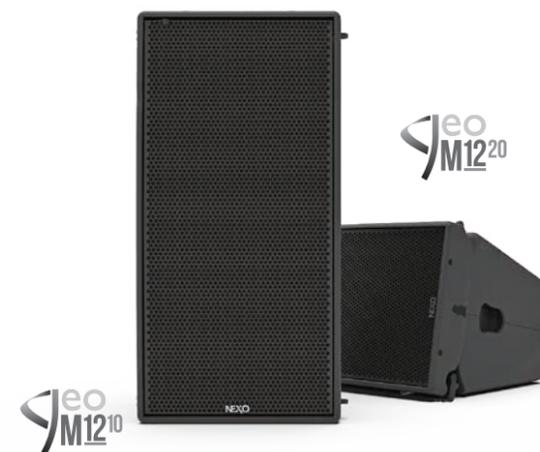
Constructed from a lightweight Polyurethane composite, the GEO M12 line array module measures 700mm wide (27.6") x 370mm high (14.6") x 446mm deep (17.6") and weighs 21kg (47lbs). It employs a 12", 8 Ohm, long excursion Neodymium driver with phase directivity device, and a 3" voice coil, 1.4" throat driver on a BEA/FEA optimised HR Wavesource™.
