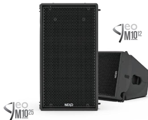
Constructed from a lightweight Polyurethane composite, the GEO M10 line array module measures 531mm wide (20.9") x 288mm high (11.3") x 355mm deep (14") and weighs 21kg (47lbs). It employs a 10", 8 Ohm, long excursion Neodymium driver with phase directivity device, and a 2.5" voice coil, 1.4" throat driver on a BEA/FEA optimized HR Wavesource™.
