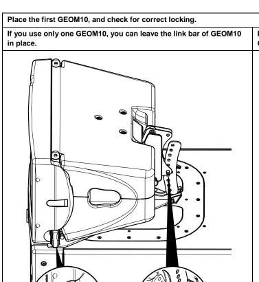
If you use more than one GEOM10, you have to get off the link bar of GEOM10 before adjusting the tilt of the first GEOM10.
