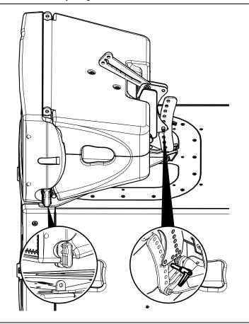
Adjust the angle between GEOM10 and MSUB15 using the Ball Lock of GEOM10 to lock the link bar of MNSTKM10 and GEOM10 (mark BUMPER and the desired angle).
