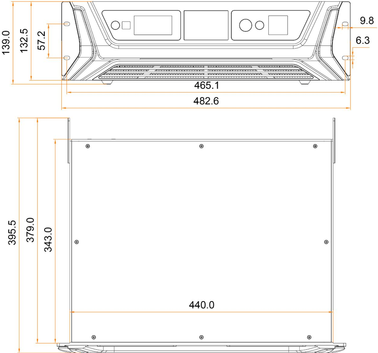
Tolerance: ±0.3 Unit: mm
