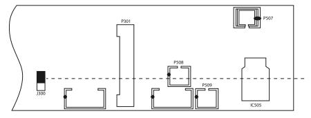
J300- MIC Emergency: Determines whether the mics remain active when an emergency signal is present at the emergency input. Default Setting: Active. Move jumper to de-activate internal mics in emergency.
