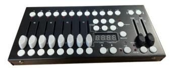
A small yet versatile 192 channel DMX controller with 12 fixtures. Each fixture controls up to 16 channels per unit. There are 23 programmable bank buttons each holding 8 scenes. These scenes can be programmed into 6 chase sequences each holding up to 240 scenes which can be triggered by sound, manually by tap or automatically by the time faders between 0.1 seconds and 10 minutes. A lightweight and portable controller, ideal for small theatres or stage applications.
