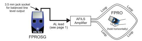
2. Switch on the amplifier and adjust the input signal control and loop drive current in accordance with the amplifier's manual.
