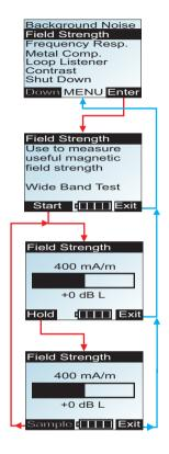
\*Note: 400 mA/m (0 dB L) is the value the AFILS must be able to produce in the usable magnetic volume to comply with EN 60118-4, but the output only needs to be 100 mA/m (-12 dB L). BS 7594:2011, clause 10 A3 (Perimeter Loops) states the field variation can be up to 6 dB L across the useful magnetic field volume, hence provided 400 mA/m (0 dB L) is achievable anywhere else in the volume of coverage, the field strength can be as low as -6 dB L (200 mA/m) elsewhere.
