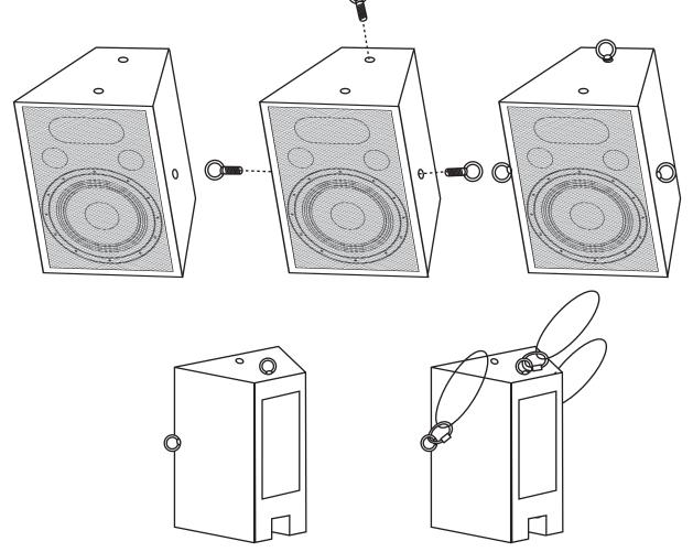
**Please note:** Before installing the eye bolts, make sure that the thread is is always in perfect condition and free from dirt.
